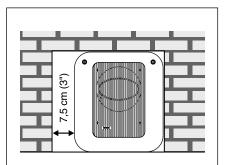
Figure 5. Flush mounting the subwoofer. Note the clearance needed on the reflex
